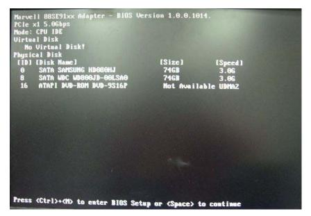
In Marvell BIOS Setup screen, select free disks to create array and continue to create virtual disk on this array. Press <Enter>.
