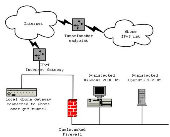
For IPv4 NAT/PAT will be used, for IPv6 routable addresses will be used, which is part of the real challenge of this setup.
